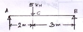
**Q6)** Determine the deflection at mid point (E) of the beam shown below by Dummy Load Method.  $EI = 2000 \text{ kN.m}^2$  [16]
